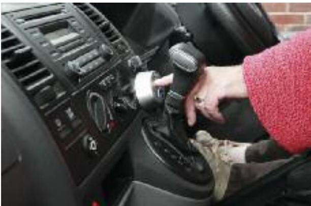
One-touch control opens door and deploys lift
