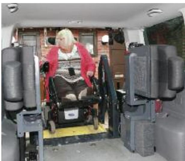
Positioning the wheelchair on the lift to exit backwards – this vehicle is fitted with folding seats in the back
