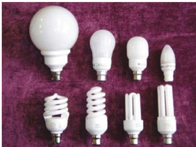
*Stick-shaped bulbs do not give much light from the end, which may make it quite dark directly under a ceiling light. Spiral bulbs are better. Enclosed bulbs (top row) have the best light distribution, but are less bright for a given wattage.*
